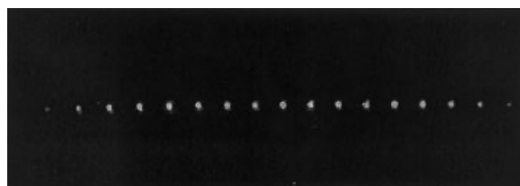
Figure 5 Real diffraction pattern of laser light through a grating spot recorded on a membrane with 1:1 (–)-BA/DP5A, 0.5 mol % RB, and 1.5 mol % NPG.
